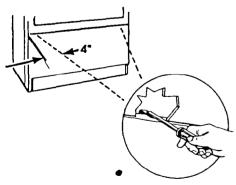
2. Remove the lower dryer access panel by releasing the two locking clips with a small, flat-blade screwdriver. The clips are located four inches in from each side of the access panel. Lift access panel off the bottom clips and set aside.
